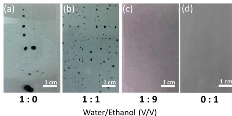
During this experiment, we searched for the best ratio between water and oil for our solvent exchange method. While increasing the quantity of ethanol from (a) to (b), the wetting/adhesion improved. Since the ethanol evaporated more quickly than the water, droplets formed while drying, leaving stains. In (c), the water evaporated at the same time as the ethanol, optimizing the drying process. A pure ethanol mixture (d) was also created, but the graphene flakes did not disperse uniformly.
