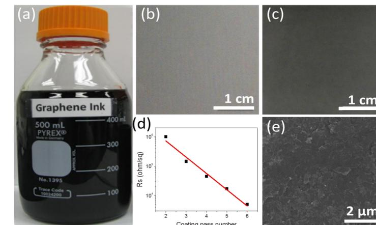
Above: (a) A picture of scalable and printable graphene ink with a volume of 500 ml transferred from NMP solution. The transfer yield is nearly 100%. Uniform graphene coating on plastic (b) and glass (c) substrates with a size of 3 cm x 3 cm, respectively. (d) Sheet resistance versus coating pass number on polyethylene terephthalate (PET) substrate. (e) SEM image of printed graphene flakes in (b).
